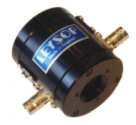
This has a modest half wave voltage (the voltage which must be applied to produce a pi radian phase shift, equal to a polarisation rotation of 90°) of around 6kV at 1064nm and has extremely high resistance to laser damage as well as being available in excellent quality crystals of large sizes. For these reasons, all our longitudinal mode Pockels cells are manufactured from >95% deuterated KD\*P.
